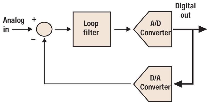
Figure 1. Block Diagram for Multibit Delta-Sigma Converter
