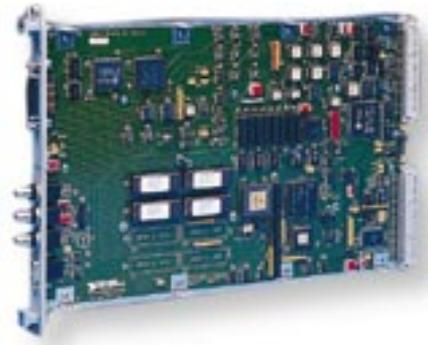
Figure 7. GPIB Controller for VXI
