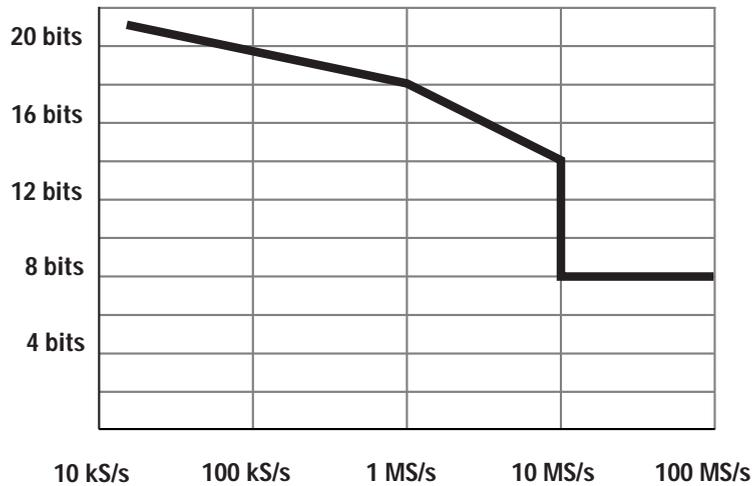
Figure 2. Flexible Resolution Sampling Rate vs Resolution
