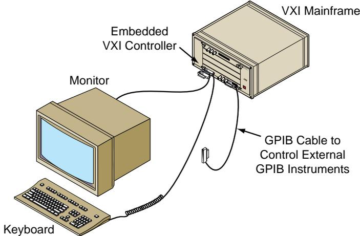
Figure 4. VXI System with Embedded Controller
