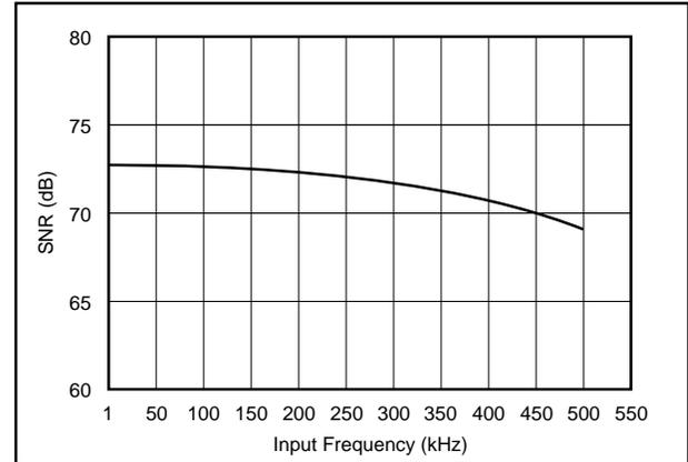
Figure 7. SNR vs Input Frequency for ADS602.
