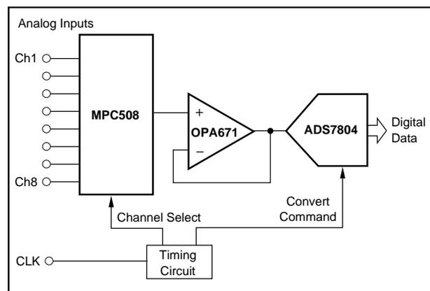
FIGURE 8. Traditional Analog Multiplexing System.
