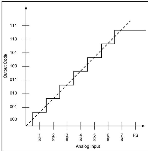
FIGURE 1. Ideal 3-Bit A/D Converter Transfer Function.
