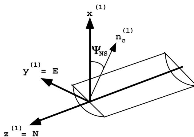
**Figure 3:** Appropriate Cartesian coordinate system for a NS-axis trough-like collector
